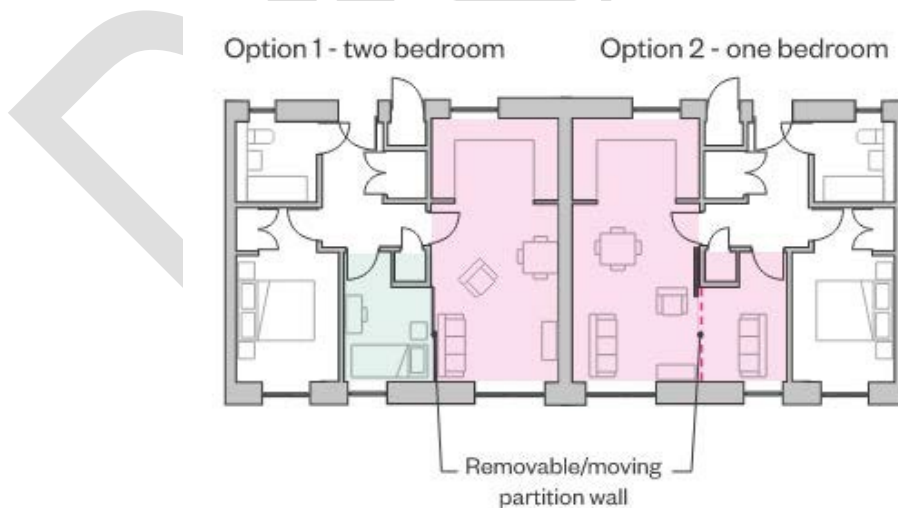
Figure 14: Design for adaptation using a flexible floor plan e.g., one bed flat can be converted to a two-bed flat or a one bed flat with space for home working.
